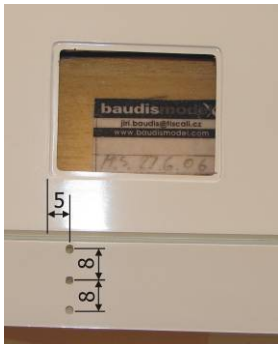
For horns drill holes 2mm
